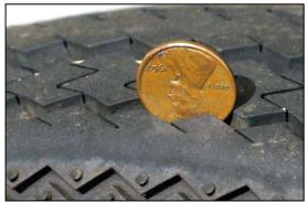
A Lincoln penny is a good measure for tread depth on both car and boat trailer tires. Place the penny upside down on the tread. If you can see the top of the president's head, the tread is worn and it's time to start looking to replace the tires **before** having tire problems.
