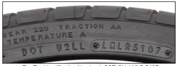
The Tire Identification Number is DOTU2LL LMLR 5107 DOT U2LL LMLR 5107: The '51' means that the tire was manufactured during the 51st week of the year 2007.
